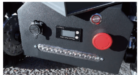
Power button, emergency brake button, battery display, LED lighting.
